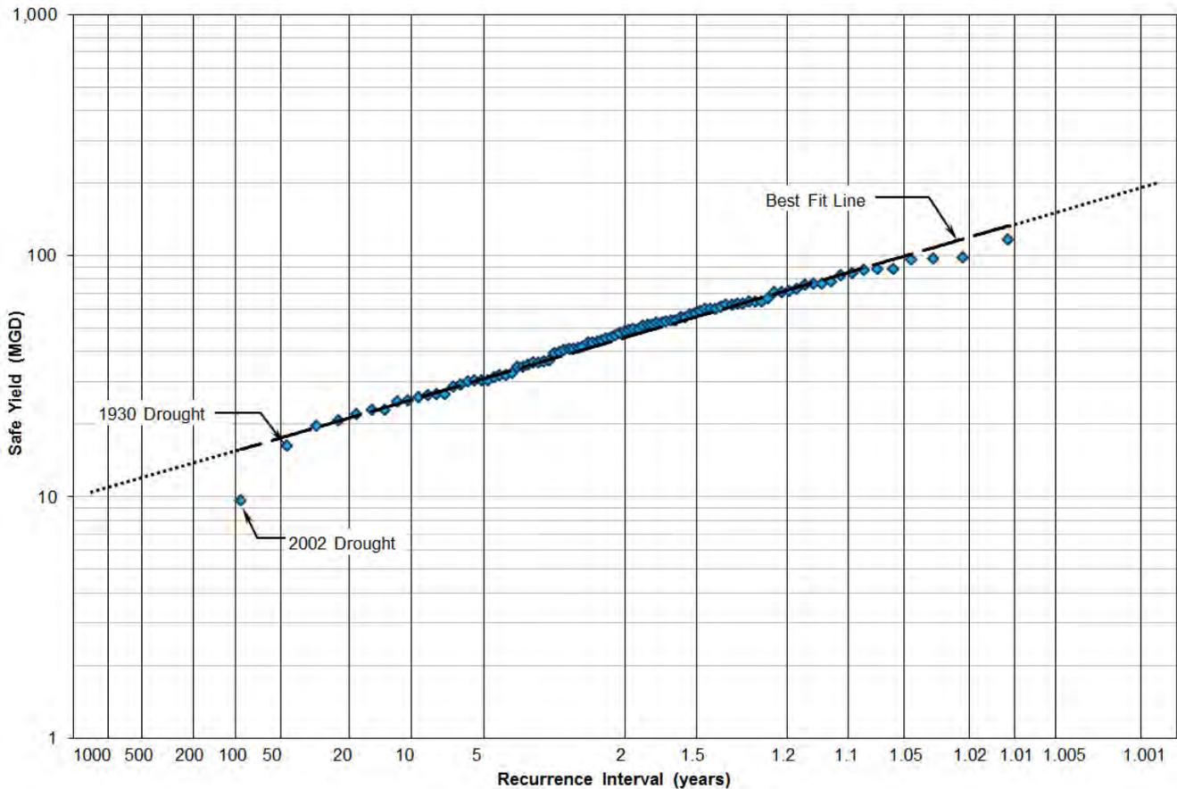
**Figure 6 – Example of Probability Plot Illustrating the Recurrence Interval of Safe Yield Values for the Entire Period of Record**
