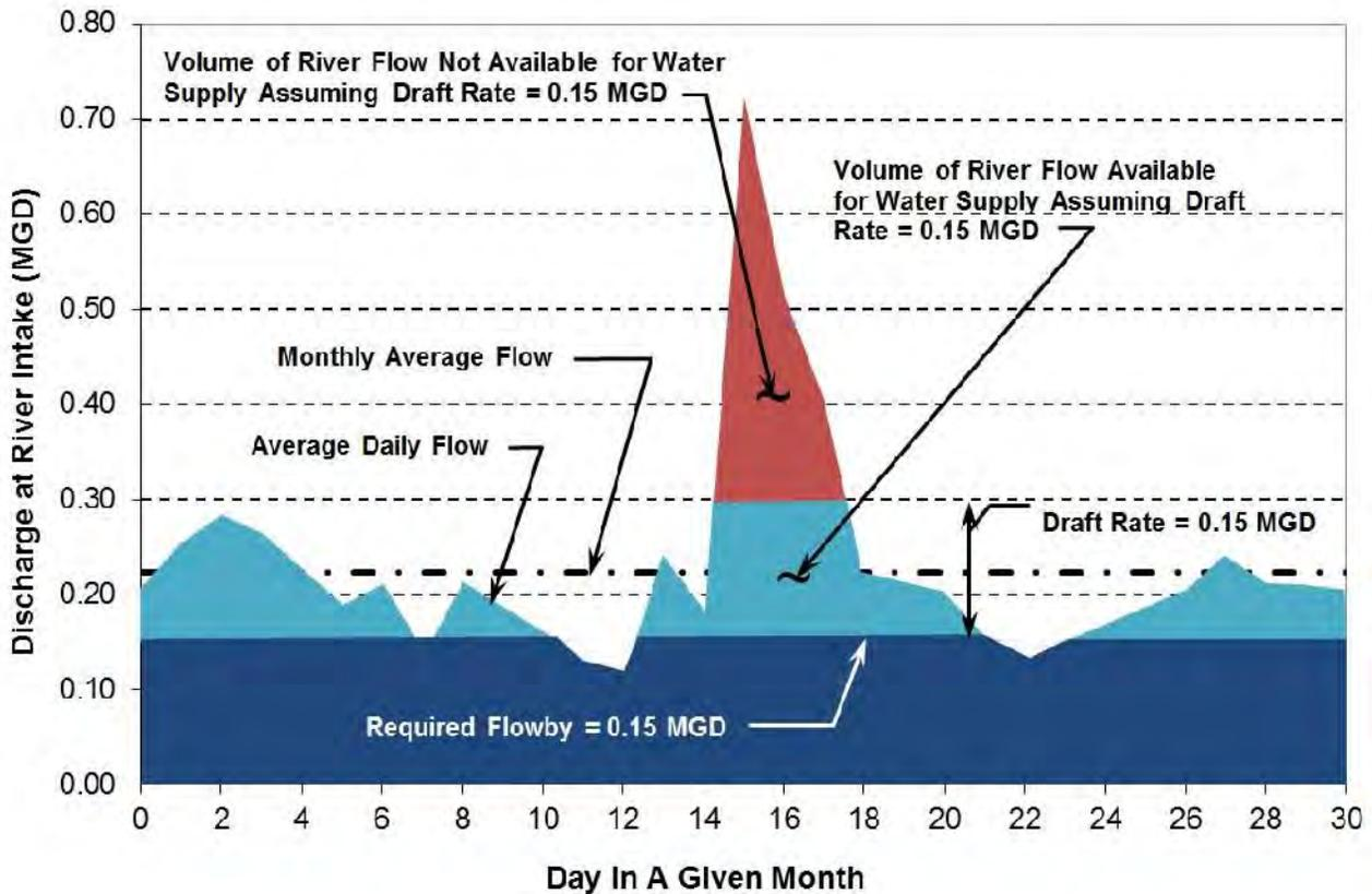
**Figure 3 – Example of Potential Overestimation of Available Source Water from a Combined River Intake and Reservoir System by Using a Monthly Time Step Instead of a Daily Time Step**
