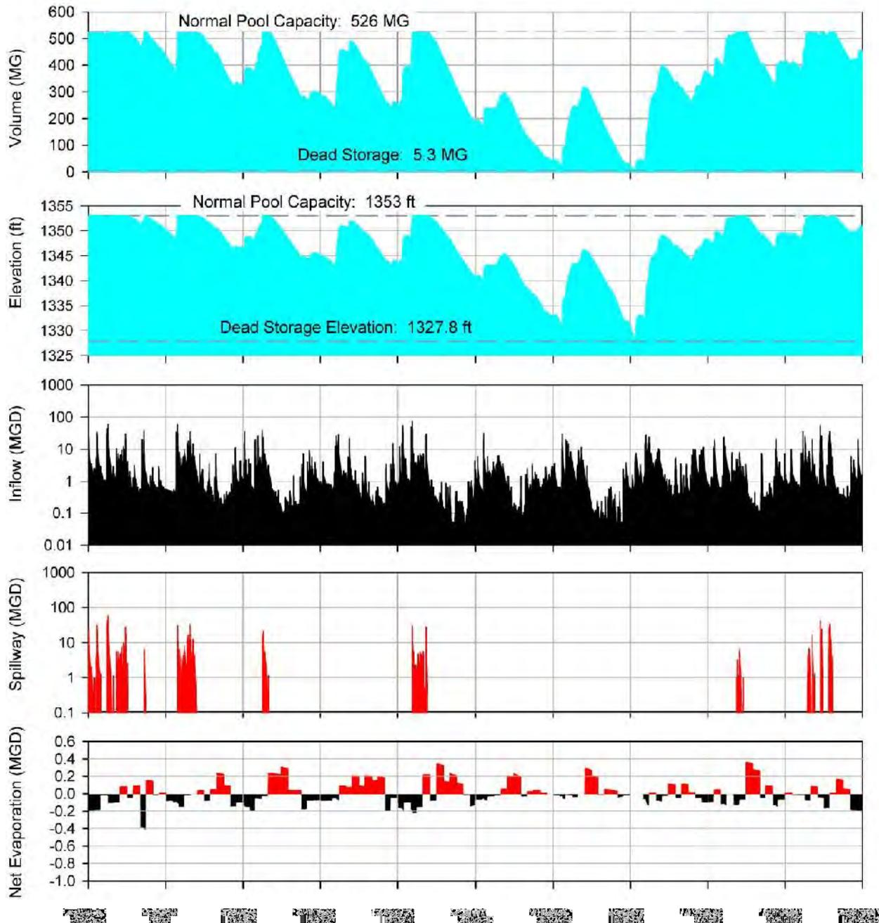
Figure 2 – Typical Graphical Output Generated from a Custom Flow Model
