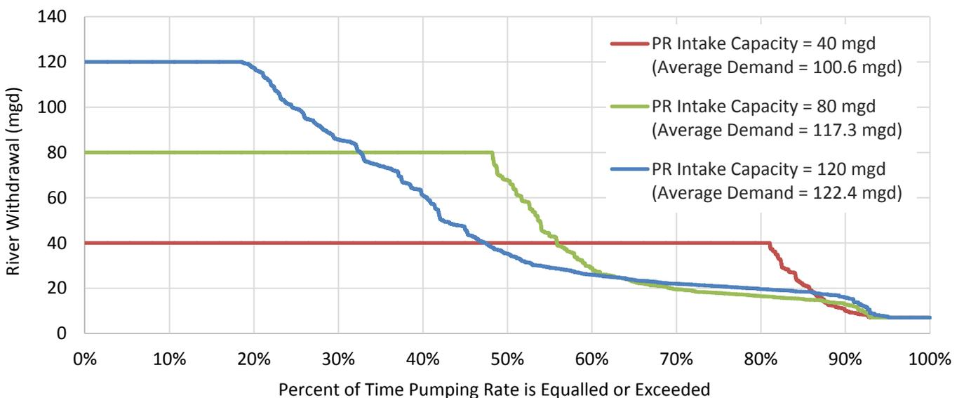
Figure 9 – Exceedance Plot of Total Withdrawals Assuming Three Varying Pump Sizes
