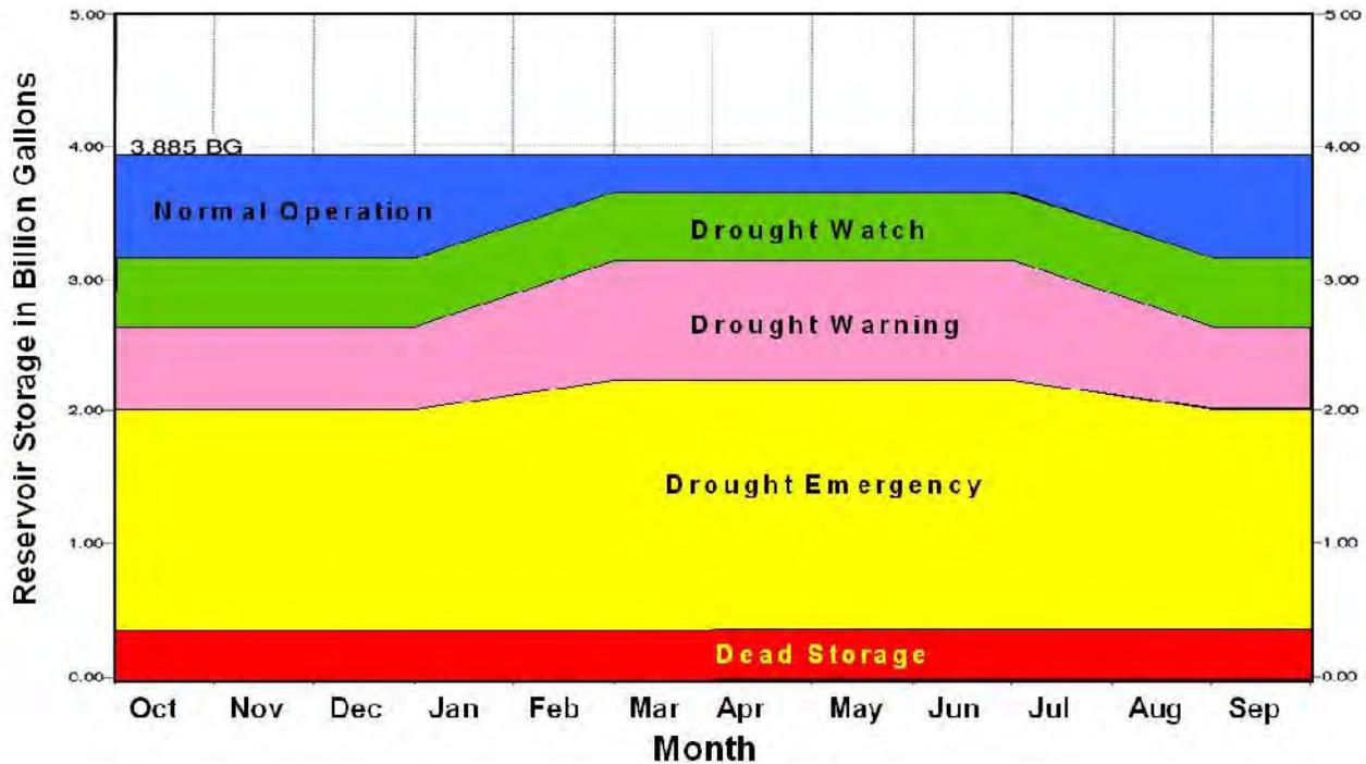
Figure 7 – Example of Reservoir Storage Condition Curves Typically Used as Part of a Drought Contingency Plan
