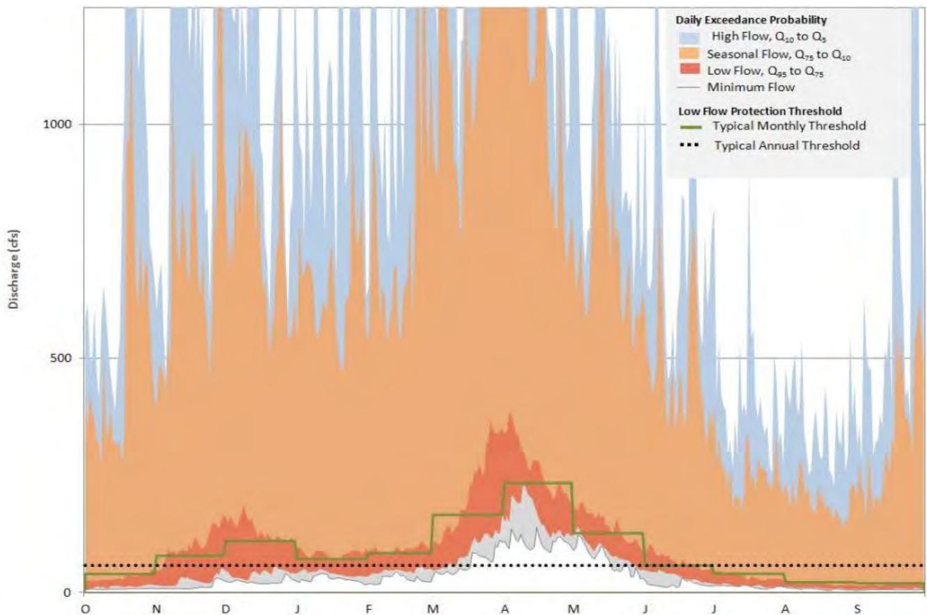
Figure 11 – SRBC Constant Annual Vs. Variable Monthly Low Flow Protection Thresholds (SRBC, 2012)
