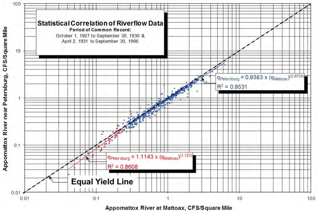
Figure 4 – Scatter Graph Showing Correlation of Monthly Streamflow Data for Two Gaging Stations
