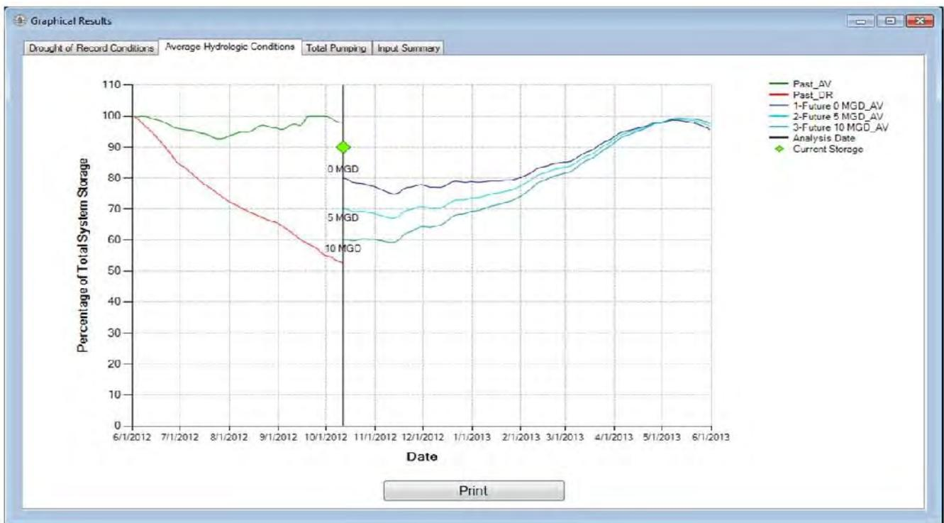
Figure 10 – Sample Application to Assist with Operating Decisions Based on Reservoir Refill Curves
