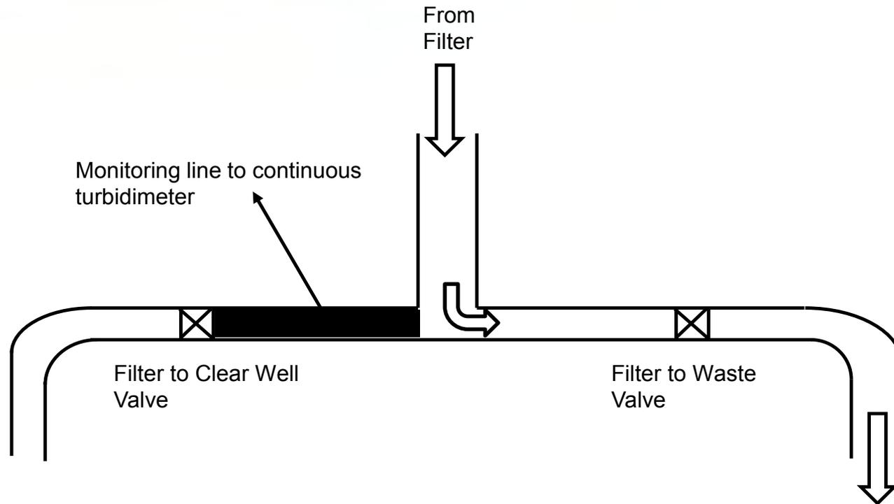
During filter-to-waste: What will be measured here?
