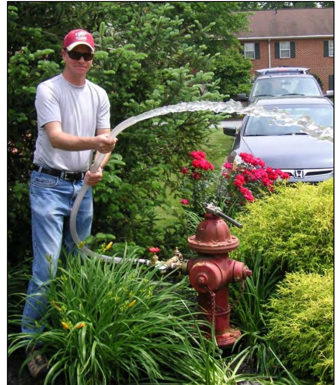
Samples collected using hydrant sampler (Sekhar & Dugan, 2009)
