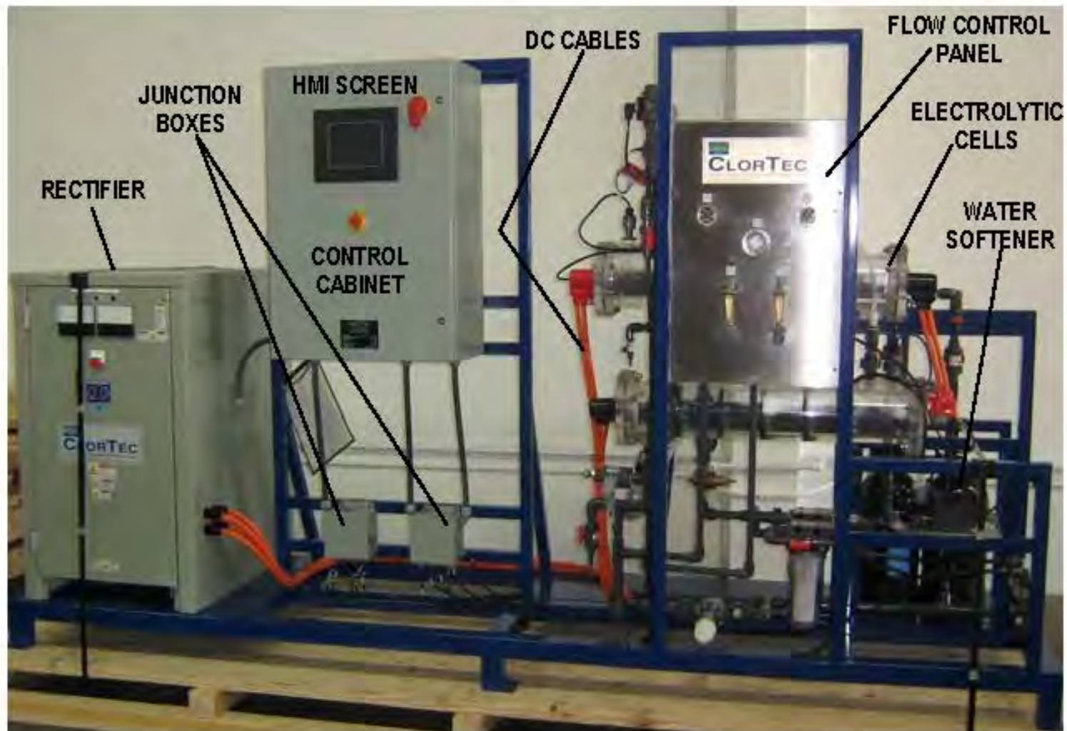
Fig. 2a - Typical medium size (CT-75 to CT-300) Hypochlorite generator system mounted on a blue powder coated skid frame
